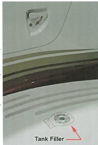
Figure 7-11 Fluid Tank Filler Location
