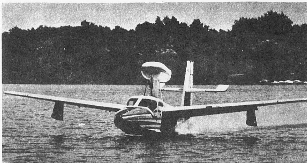
TAKE-OFF FROM WATER requires practice. Flaps may be left up until plane is on the step and then lowered. Pilots must be alert for changes in plane attitude and for obstructions on the water.
